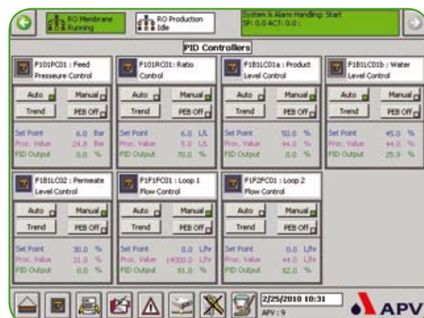
PID control screen for easy and quick access to PID control loops
