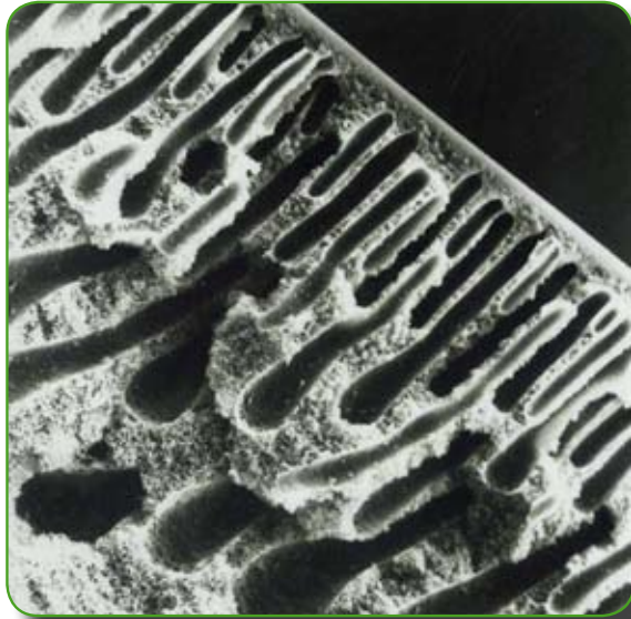
Fig. 12: Close-up of a UF membrane
