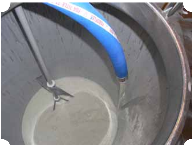
Fig. 4: Cleaning test on a process tank soiled with yoghurt milk. The cleaning procedure was mild caustic cleaning followed by 43 ppm HOCL cleaning. The soiled tank is on the left and the completely clean tank after cleaning is on the right
